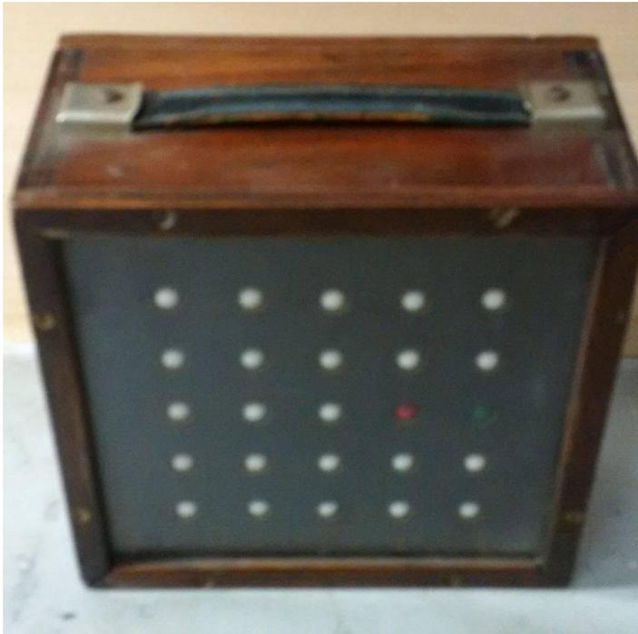
Used on the Training Group in 1966, to train us apprentices how Sampling works. It contains 100 balls, of which 10 were green, to represent minor faults and 5 which were red, to represent major faults. A shake and then held upside down, it would randomly display 25 of the balls. Given enough samples, you could work out the number of red & green balls that were in the box. I remember that it made my arms ache!
